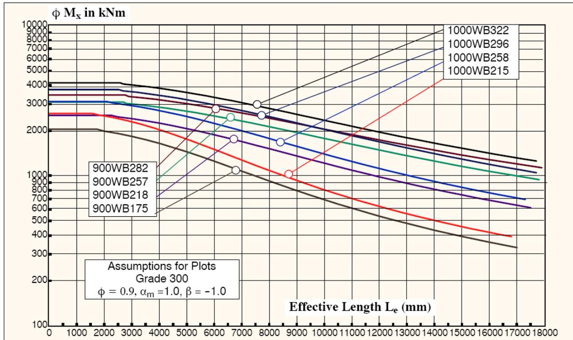
Figure 3-2: Design member Moment capacity  $\phi M_b$  [kNm]. (Doh, 2006)
