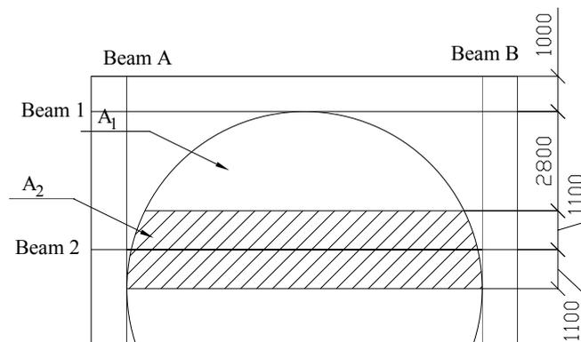
**Figure 3-1:** Spacing of beams, all measures in mm.
