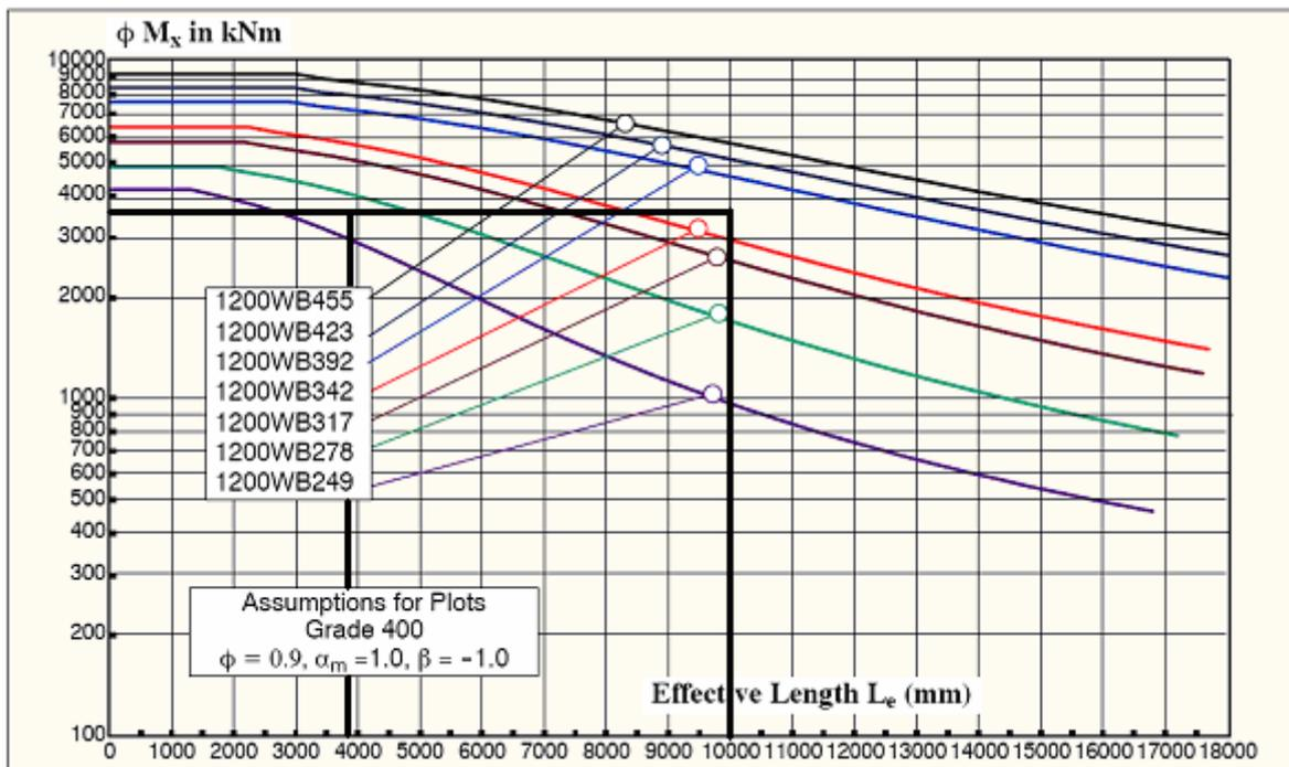
**Figure 3-3:** Design member Moment capacity  $\phi M_b$  [kNm]. (Doh, 2006)
